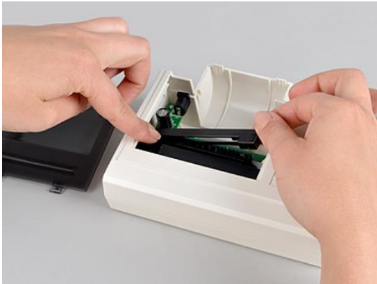
Fig. 15: Inserting the ink ribbon
