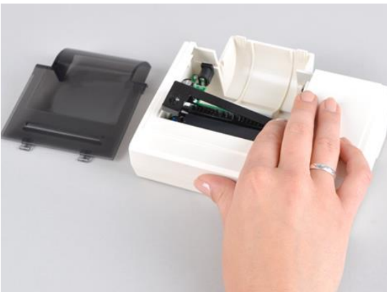
Fig. 14: Removing the ink ribbon
