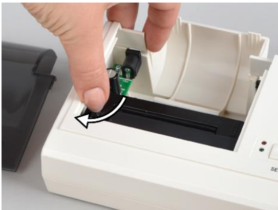
Fig. 16: Tightening the ink ribbon k
