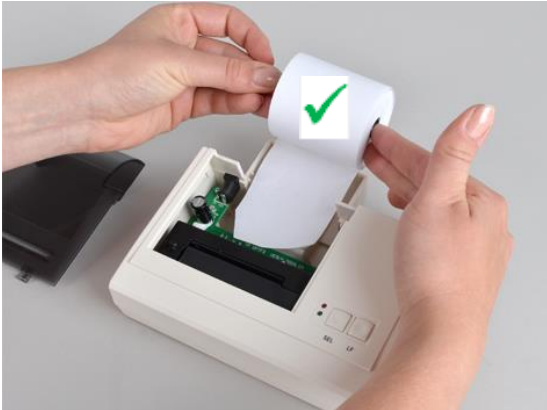
Fig. 8: Inserting the paper roll correctly
